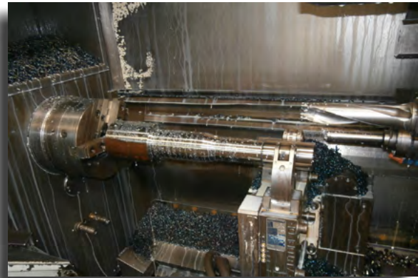
MACHINING CNC machining centers Drilling of one-piece solid cylinder
